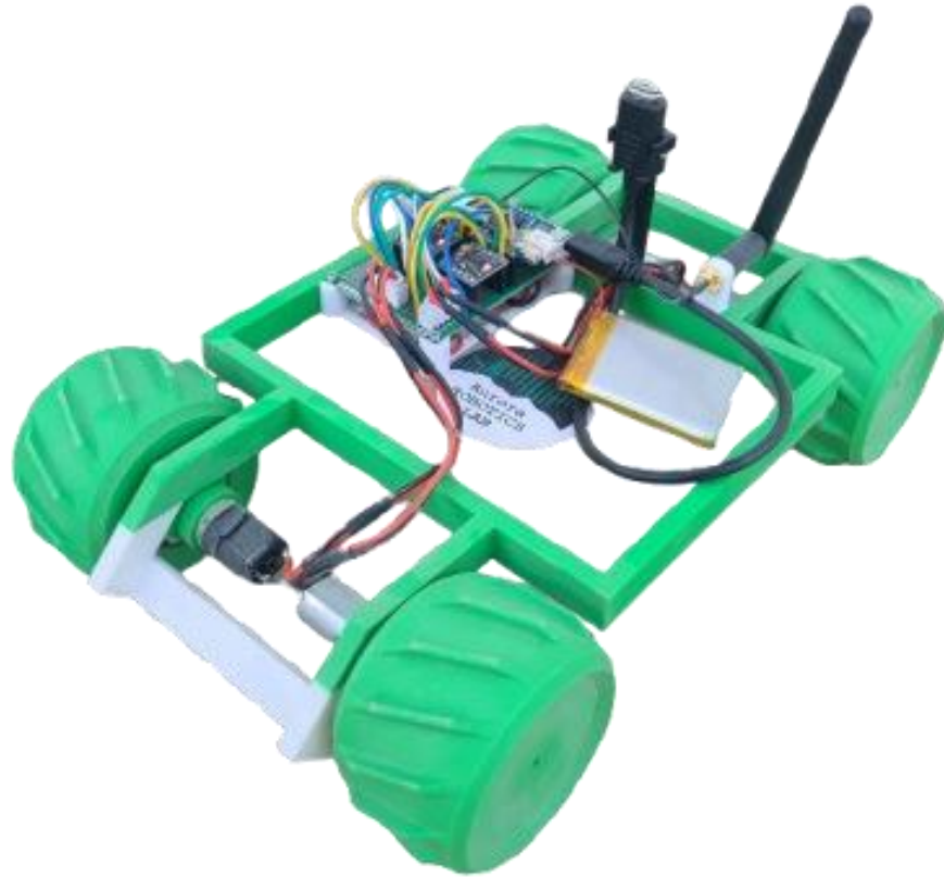
Figure 3.4: MiniLAMP, an MCU-based Pebble platform.
