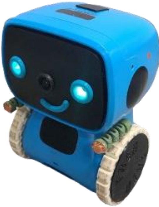
Figure 3.3: Fred, a Pebble platform built on a commercial toy base.
